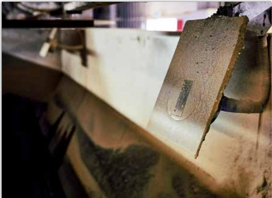
*Solitrend ensures fast and reliable measurement of moisture directly in bulk solid flows.*
