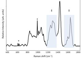
Figure 2: The Raman spectrum of a plant-based protein provides information on composition (\*) and molecular structure (highlighted in grey).
