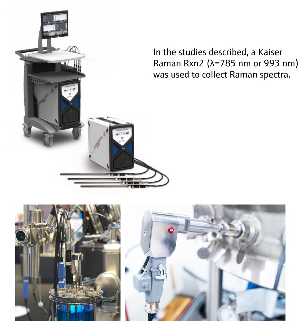
*In situ* bioprocess monitoring achieved using Kaiser probes for lab-scale/PD (bIO-Optic, left) or manufacturing scale (bIO-PRO, right) in single-use, glass or stainless steel bioreactors.
