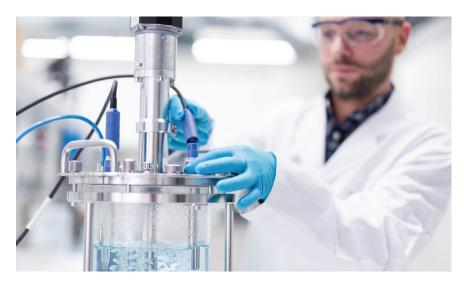
The oxygen consumption depends on the cell type and its concentration in the bioreactor. How well, healthy and quick the cells can grow has to do with our ability to deliver oxygen to the cells. The rate of transfer of the oxygen in solution and the rate of the oxygen consumption by the cell are of highly importance.
