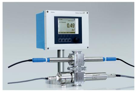
Cleaning In Place (CIP) and Sterilization In Place (SIP) do not have any impact. The 4-pole conductivity sensor is easy to calibrate in the lab or in the workshop, thanks to the Memosens technology combined with the use of Memobase Plus CYZ71D-software. The software is suitable for use in GLP/GMP- work environments.
