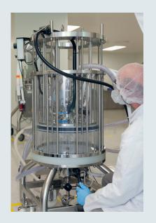
The fermentation is performed in the upstream process. The product is then ready for the downstream process which includes a number of steps. The first step is the primary recovery, followed by initial purification, polishing, and finally the formulation.
