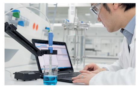
A crucial activity during fermentation is the control of the acidity of the culture medium which is measured by the indispensable pH sensor.
