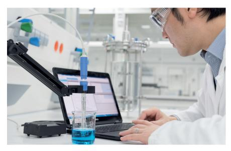
A crucial activity during fermentation is the control of the acidity of the culture medium which is measured by the indispensable pH sensor.
